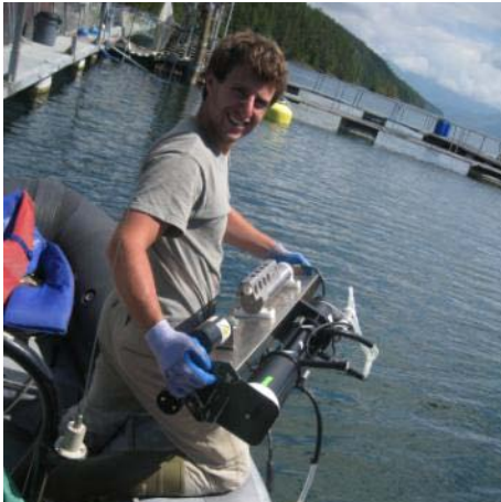
Justin Del Bel Belluz holding a hyperspectral attenuation and absorption meter.
